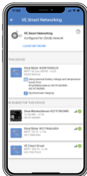
Example of a VE.Smart Networking
